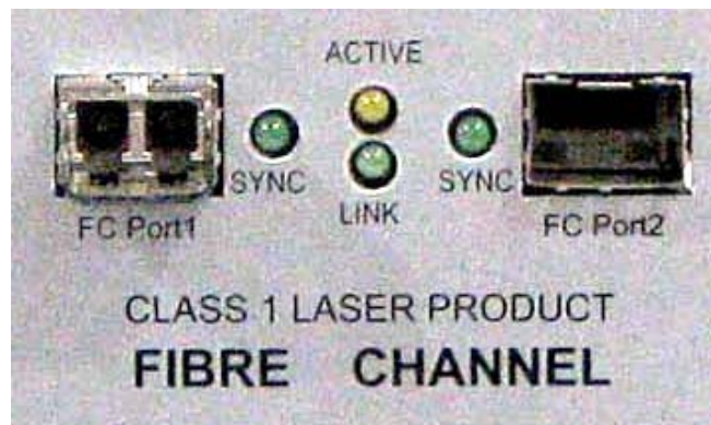
FIGURE 4-5. Built-In Hub, Showing the LEDs Located Between the Fibre Channels.
